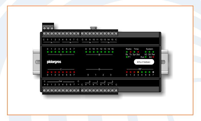
The RTU-710H/DA1 is remote I/O module with on-off, analog inputs and on-off outputs. Event counting and time totalizing functions can be enabled for on-off inputs. An optional PicoLogo Micro-PLC feature allows the RTU-710H/DA1 to act as an autonomous micro-PLC. All I/Os are electrically isolated from the module's electronic circuits.
